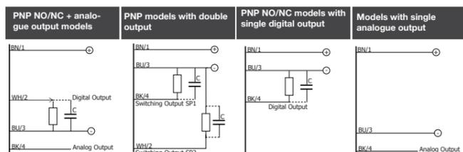
In case of combined load, resistive and capacitive, the maximum admissible capacity (C) is 0,1 µF for maximum output voltage and current.
